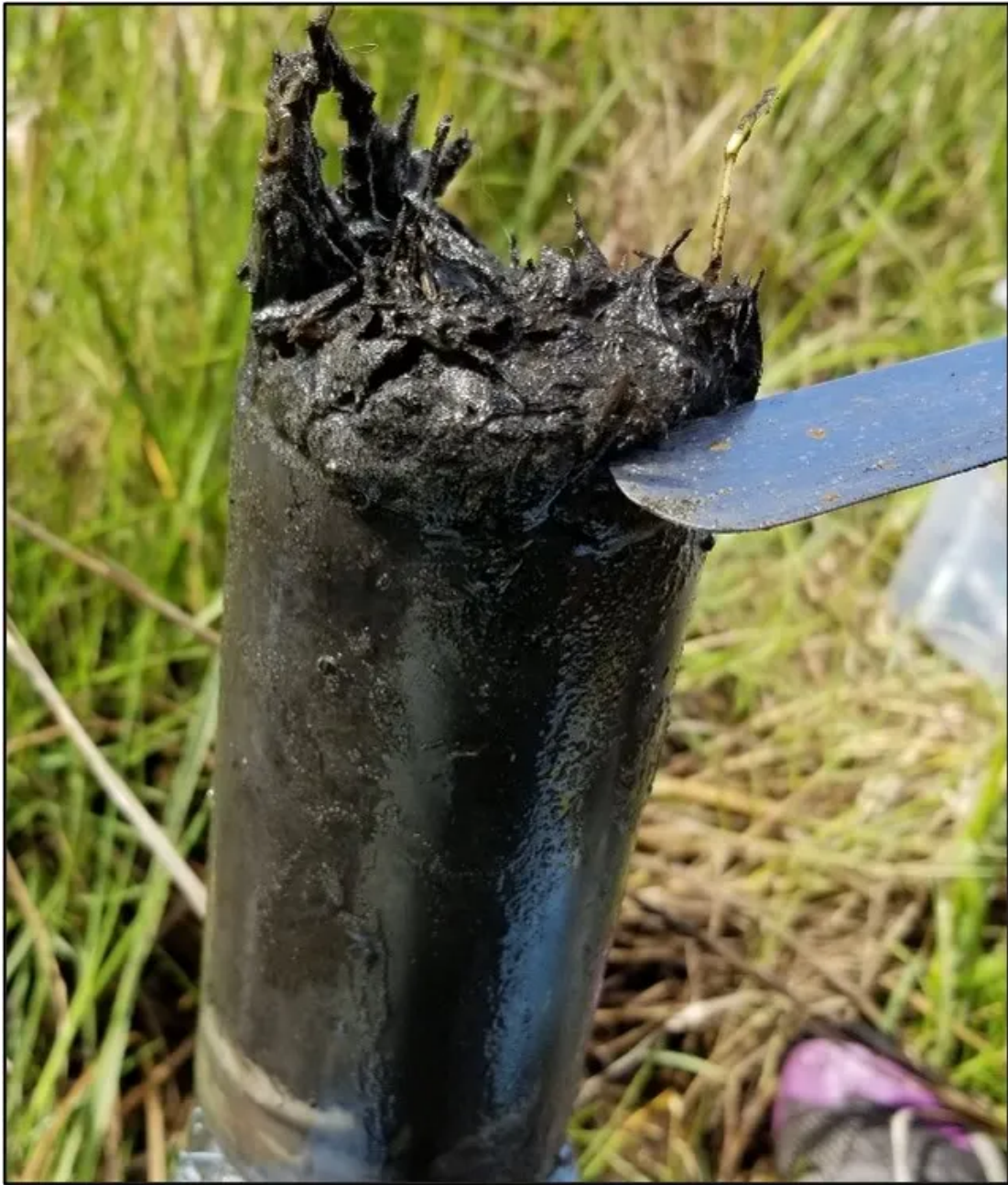
Natural marsh soil core, showing black color, predominately clay content mixed with organic matter.
